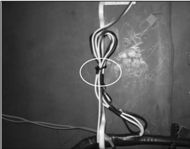
Fix DGC lead wire to DGC band using a 9mm purple lock (3-703-982-02)
