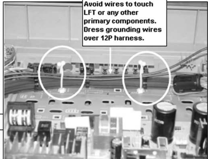
On HU purple locks CLS1006 and CLS1007 (4-049-278-01 x 2) dress 12P harness (M~HM) and A~HM board grounding wires.
