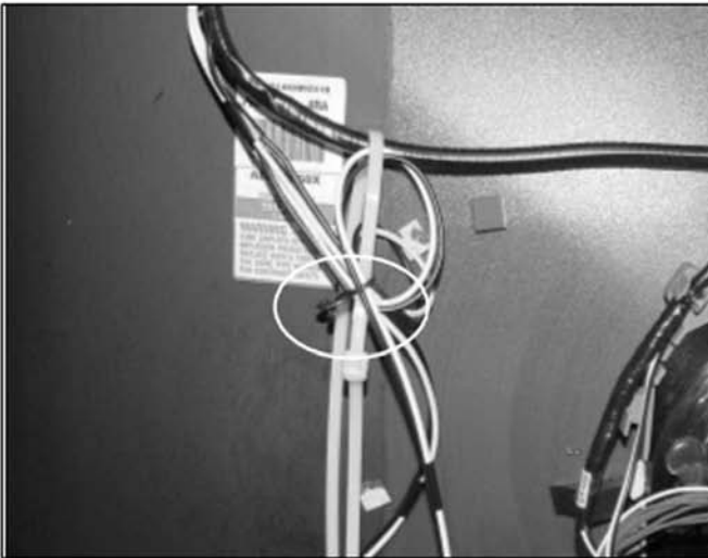
Dress DGC lead wire using a 9mm purse lock (3-703-982-02).
